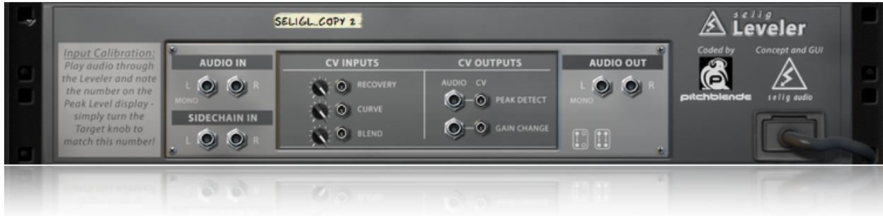
Here you will find all the I/O for the Selig Leveler. Naturally there are audio inputs and outputs, as well as a side chain input. Also included are CV inputs for the Recovery, Curve, and Blend controls, and CV and audio level outputs for the Peak Detector and Gain Change circuits. For easy reference, the calibration instructions are located on the left side of the back panel.
